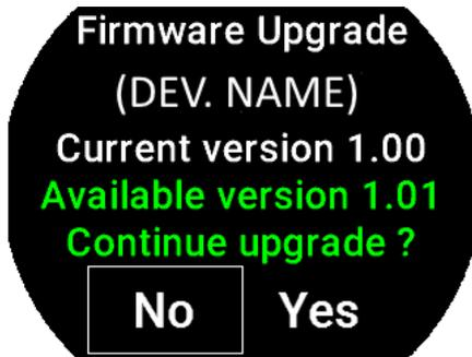
In case you are installing a version prior to the installed one, a different message will inform that you are **downgrading** and not upgrading the software. Confirm “Yes” to proceed, “No” to exit without writing any software.
