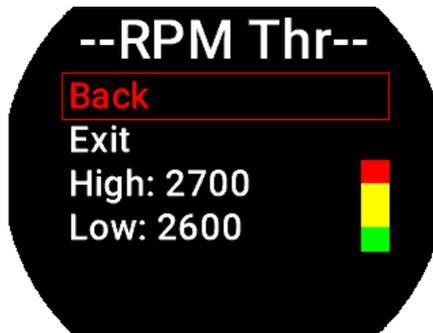
Rotate the knob to highlight the threshold you want to change, push and change the value, push again to confirm. Default thresholds are at 0.
