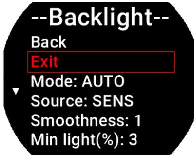
**Source:** choose "Sens" to read the brightness from the optional sensor connected to the instrument itself or "CAN" to read the ambient brightness from the CAN1 bus if the brightness sensor is connected to another **Omnia** instrument connected in cluster.
