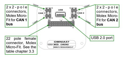
The required connectors and terminals are supplied with the instrument
