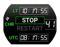
To stop the chronometer, press the knob, rotate it and confirm "STOP", the elapsed time will remain on the screen. To count the time again repeat the procedure above.
