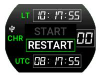
When the chronometer is stopped at any value, press the knob and confirm "START" to restart the count from the previous value or press "RESTART" instead to have it count again from zero.
