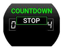
To stop the COUNTDOWN, click the knob and confirm "STOP". The previous set time value will be recalled. Not choosing a function within 5 seconds will cause the menu to disappear.
