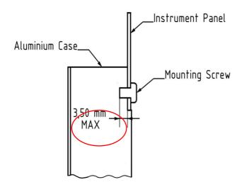
The screws supplied (M4x6mm), are suitable for panel thicknesses between 1.5 mm and 2 mm.
