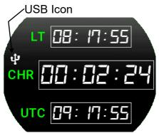
To activate the Logger choose "Yes" from the Main Menu>Logger. The icon will turn **green** when the file is being written and **red** when the Logger is enabled but the USB stick is not connected or in case of writing problems.
