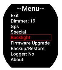
**Exit:** confirm to "exit" from the setup menu and go back to the main screen.
