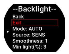
**Source:** choose "Sens" to read the brightness from the optional sensor connected to the instrument itself or "CAN" to read the ambient brightness from the CAN1 bus if the brightness sensor is connected to another **Omnia** instrument connected in cluster.
