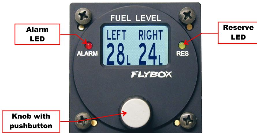
The knob can be rotated or used as a pushbutton (for example it must be rotated to increment or decrement a value and pushed to confirm).
