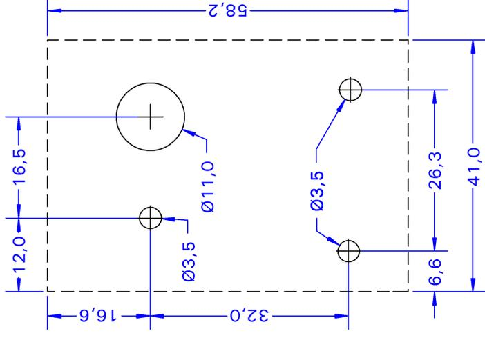
**NOTE: don't enter with the screw thread more than 6mm inside the panels**
