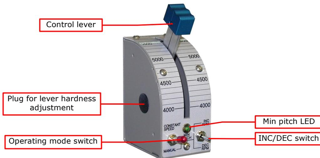
**The operating mode switch has a safety lock to avoid accidental operation: it must first pulled on the outside and then moved to the desired position.**
