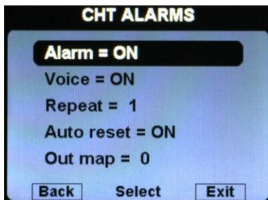
● **Alarm = ON/OFF:** enable/disable the alarm (alert indication on display) that occurs when a CHT measurement exceeds the red threshold (default=ON).
