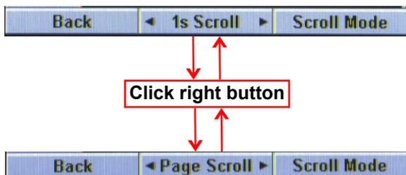
With the “1s scroll” mode, rotating the knob move the cursor by 1 step (that is 1 second of flight record); with the “Page scroll” mode, rotating the knob move the cursor by 1 page (so it works as a fast forward/rewind).
