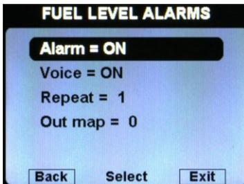
**Alarm = ON/OFF:** enable/disable the alarm (alert indication on display) for the low fuel on any of the available tanks (default=ON).
