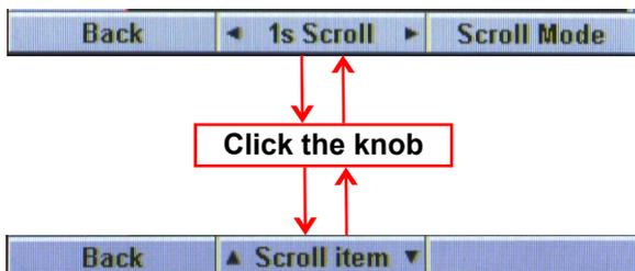
When this mode is active, rotate the knob to scroll through the item/measurements available; click again the knob to go back to the cursor scroll mode.
