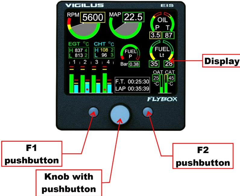
The knob with pushbutton can be rotated (for example to increment or decrement a value) or pressed like a pushbutton (for example to enter in a submenu).
