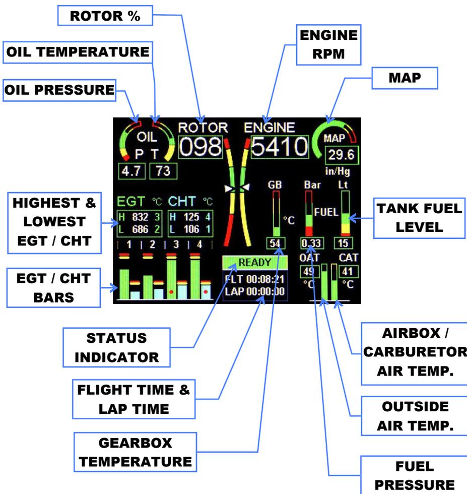
On this page all the important engine data is clearly displayed in both graphical and numerical indications. The green, yellow and red zones of the various gauges is completely customizable as explained in chap.1.3.4 “Instruments menu”; when a measurement is on a yellow or red zone the corresponding numerical indication change color to yellow or red; when in red zone the corresponding gauge is also blinking.
