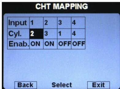
Since the Rotax engines are provided with two CHT sensors, but the first is for the cylinder#2 and the second is for the cylinder#3, this configuration make sure that the first input of the remote module (where is connected the first sensor) is referred to the cylinder#2, while the second input of the remote module (where is connected the second sensor) is referred to the cylinder#3; the third and fourth inputs are disabled (Enab. = OFF).
