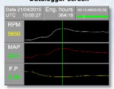
All data are recorded and stored in memory for over 200 hours of recording. The data can be viewed directly on the display or downloaded for viewing and archiving on a PC.
