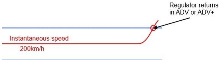
In the image above, the speed increased to the upper Speed Window limit of 220 Km/h and the APR1 controller returned to ADV or ADV+ mode, indicating this on the display.
