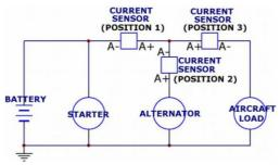
**Position 1:** the current sensor measure current flow into or out of your battery (indicator show both positive and negative currents).
