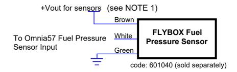
**NOTE 1:** use sensors which support the voltage supplied to PIN 1 only.
