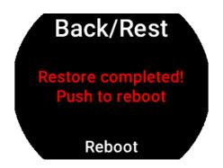
Push the knob to reboot, the new parameters are now loaded in the instrument.
