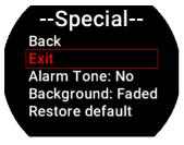
Alarm Tone: choose "Yes" only if the alarm output will be connected to the optional Flybox "Audio Tone Adapter". This way the output generates a high-pitched tone instead of a continuous signal.
