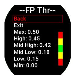
**Thresholds:** set all the thresholds for the Fuel Pressure gauge.
