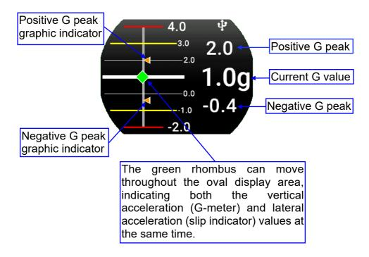
During the flight, if a set threshold is exceeded, the alarm related to that threshold will appear on the screen and the alarm output will be activated.
