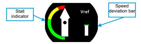
The figure represents the indicator when the aircraft is stationary on the ground. The stall indicator arrow is at the end of the red arc because the lift is at zero, while on the right of the screen, the speed deviation bar of the Vref is shown.
