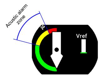
While cruising or at a speed significantly higher than the stall speed, the indication will be as in the figure. As the stall speed approaches, the white arrow will begin to move towards the yellow section of the arc, upon reaching it, the alarm output will begin to emit tones that will become closer and closer as the arrow moves towards the red arc. As soon as the arrow touches the red, the tone becomes a continuous sound.
