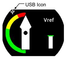
To activate the Logger choose "Yes" from the Main Menu>Logger. The icon will turn **green** when the file is being written and **red** when the Logger is enabled but the USB stick is not connected or in case of writing problems.
