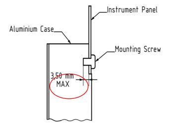
The screws supplied (M4x6mm), are suitable for panel thicknesses between 1.5 mm and 2 mm.
