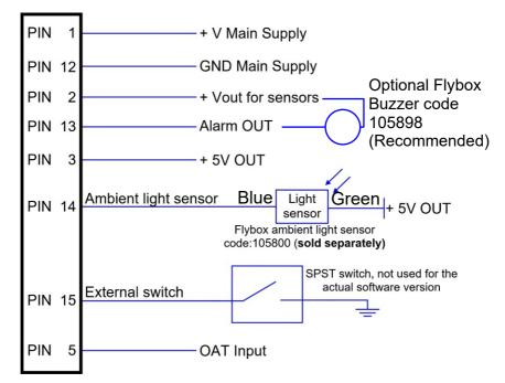
It is strongly recommended to use the dedicated buzzer, Flybox code 105898. Using an external buzzer ensures that the alarm signal is never filtered out by intercom or radio settings as it is completely isolated from them.
