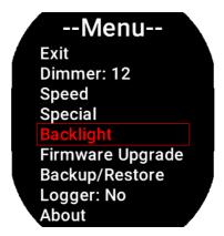
**Exit:** confirm to "exit" from the setup menu and go back to the main screen.
