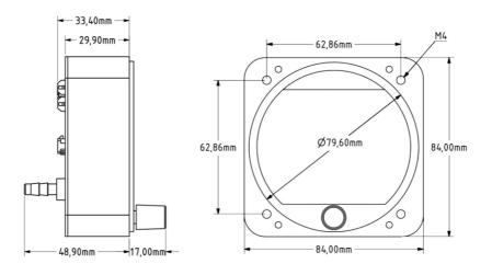
**NOTE:** For an installation without interference, consider making a hole of at least 80.5 mm diameter.
